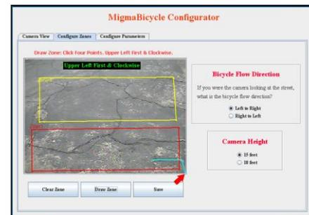
**Step 6:** Finally touch the lower left corner. Observe that the zone is complete.
